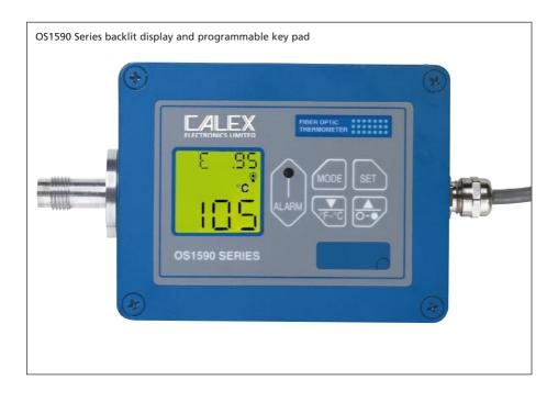
The unit provides two separate analogue outputs. The first is 1mV/Deg. The second is specified -\* , where: - mA = 4-20 mA output; - V1 = 0/5 Vdc output; - V2 = 0/10 Vdc output; - K = 1 Thermocouple output, K = 1 Thermocouple output,
